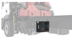
ÖLK02 - Oil cooler 10,5kW, loose Longer service life of the oil, seals, valves and other hydraulic components through lower oil temperature
